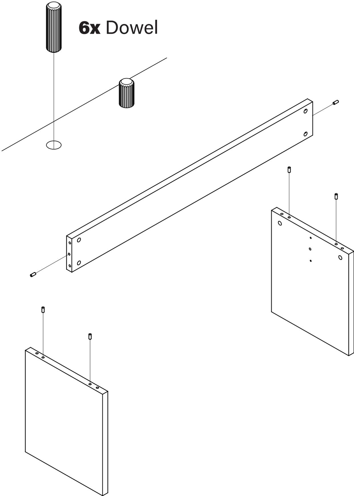
**Place the 6x Dowels in respective holes of the crossbar and legs.**
