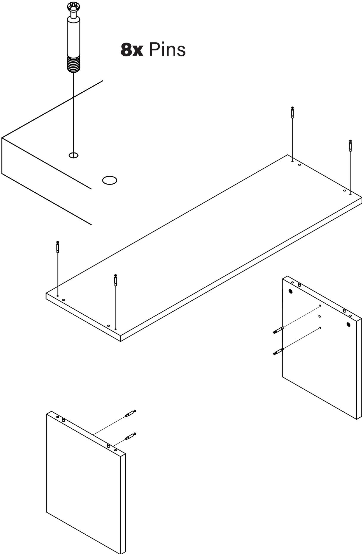
**Now the 8x Pins have to be attached to the backside of the bench seat and the legs.**
